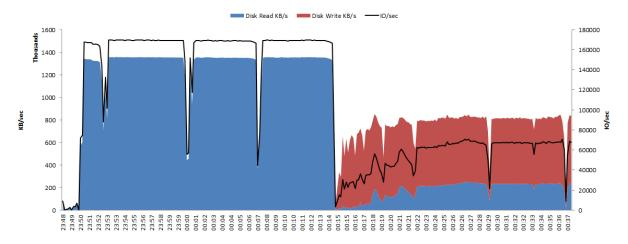
These figures indicate a maximum IOPS of 168997.3 to generate 1351975.9 kb read/s during the reader test. The peak for reads was 586326.1 kb written/s, 232419.1 kb read/s at 67169.3 IOPS. Again, the dip in the centre is the change from reader to writer test, when the next series of tests commenced.
