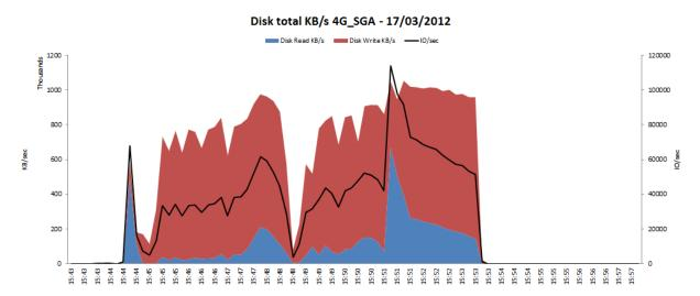
The dip in performance is due to the start of the second test series-there was no problem with the card.
