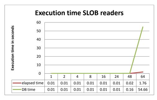
The red line is execution time as measured by the wall clock. AWR reports it as 1 second, rounded up, except for the 64 readers-case where it is 1.76 seconds. The DB time in the last scenario went up to 31 seconds. Try this with your storage!
